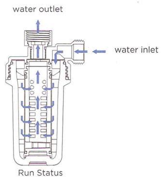
Raw water from the water inlet, through the built-in stainless steel mesh, filter out the rust in the water, sediment and other large particulate matter, make preliminary purification of the water quality, protecting the back-end water equipment.
